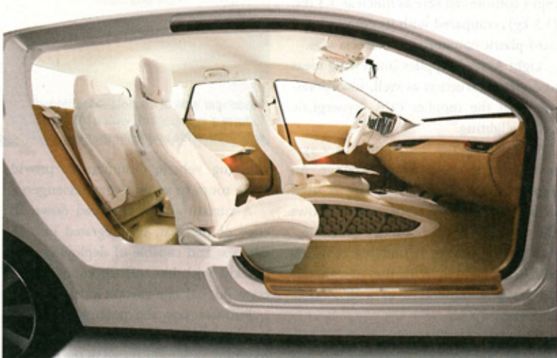
"Seat-wing" control module positioned atop center console for driver's easy access. Battery cells appear below center console.
