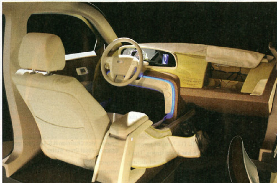
Light Attitude's glove box "door" is actually a piece of fabric that pulls back like a blanket to reveal storage space.
